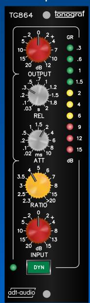
The TG864 is a fixed threshold low noise FET-Compressor with the typical fast and aggresive characteristics of FET based compressors. The control circuit uses handpicked FETs and a complex distortion compensation.
